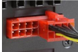
You can connect 1 or 2 modular 8-pin cables into any of the 16-pin sockets
