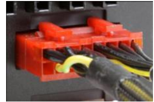
You can connect 1 or 2 modular 8-pin cables into any of the 16-pin sockets
