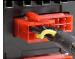
You can connect 1 or 2 modular 8-pin cables into any of the 16-pin sockets
