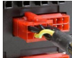
You can connect 1 or 2 modular 8-pin cables into any of the 16-pin sockets
