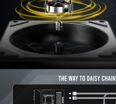
Hydro bearing PC case fans operate at noise levels  $\leq 29$  dB(A), ensuring a quiet computing environment while offering smoother, quieter operation and enhanced durability (30,000 hours) by reducing friction and wear.
