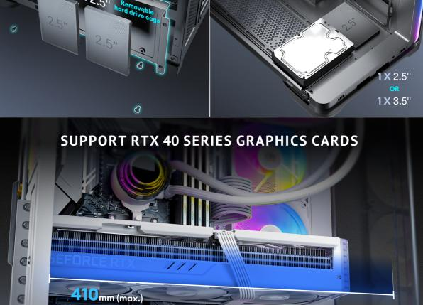
Removable hard drive cage provides space for 1 x 3.5" HDD and 2 x 2.5" SSD. The case bottom can additionally accommodate a 3.5" HDD after removing the frontmost bottom fan, or a 2.5" SSD after removing the lowest side fan.
