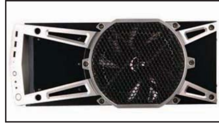
Massive cooling system highlighted by top 200 mm fan
